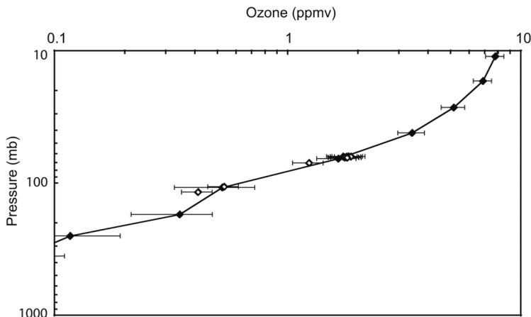
**Fig. 4.** Ozone mixing ratio measured by MIPAS-E (v.4.61) at 09:19:25 UTC, (45.7° N, 12.9°E), error =  $\pm 3\sigma$  (black diamonds) and GASCOD/A4 $\pi$  (open diamonds) around (45.2°N, 10.2E) zone. Data are obtained during APE-ENVISAT Mid-Latitude Campaign held at Forlì airport, flight 22 July 2003.
