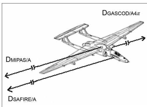
**Fig. 1.** Observational directions of MIPAS/A, GASCOD/A4 $\pi$  and SAFIRE/A instruments aboard M55-Geophysica aircraft. Measured parameters are assigned to areas of ~150 km±300 km away the aircraft (MIPAS/A and SAFIRE/A) and ~50 km±70 km (GASCOD/A4 $\pi$ ).
