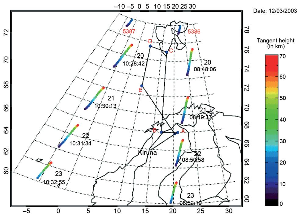
**Fig. 2.** M55-Geophysica aircraft flight route (12/03/2003). MIPAS-E scan 21, orbit 5386 (08:49:37UTC) is compared to GASCOD/A4 $\pi$  measurements. Closest correlation corresponds to EA back leg around 69N+71N (see fig. 3). Color bar indicates the tangent height of MIPAS-E line of sight.
