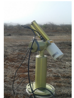
Right below: Cimel (right) sunphotometers deployed at Praia
