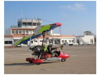
GAMARF TA campaign: The IMK-IFU ultralight aircraft D-MIFU, instrumented for airborne aerosol and radiation research, during its take off at Lampedusa airport. The airborne instruments allowed for the measuring of the longwave irradiance profiles for the first time in the Mediterranean.
