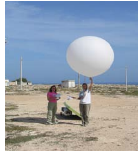
GAMARF TA campaign: two ENEA researchers during a radiosonde launch. The information from the radio sounding was used to integrate the ground-based and airborne measurements.
