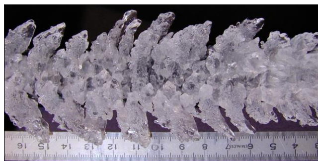
Ice deposits on a wing obtained in a wind
