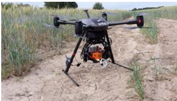
COSI camera mounted on a drone
