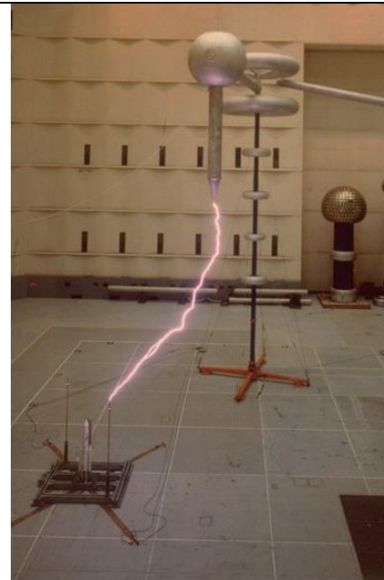
Artificially simulated lightning onto a model of the Ariane 5 rocket launch pad.
