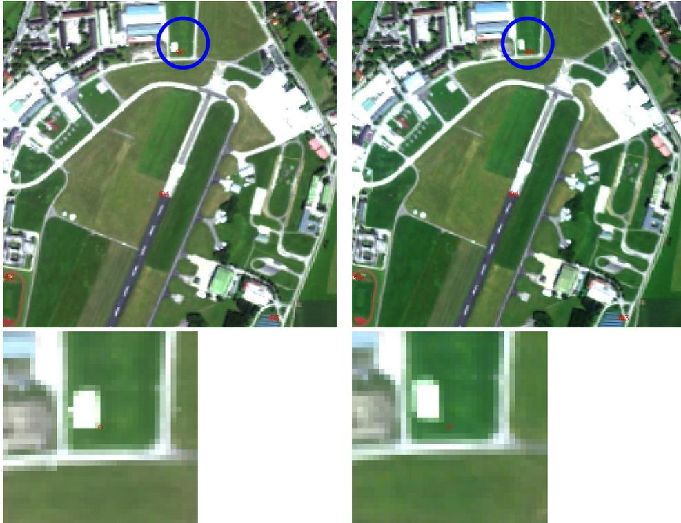
Figure 3: Results of geometrically corrected HyMap data (Kaufbeuren 2009) with PARGE (left) and ORTHO (right): Direct comparison.
