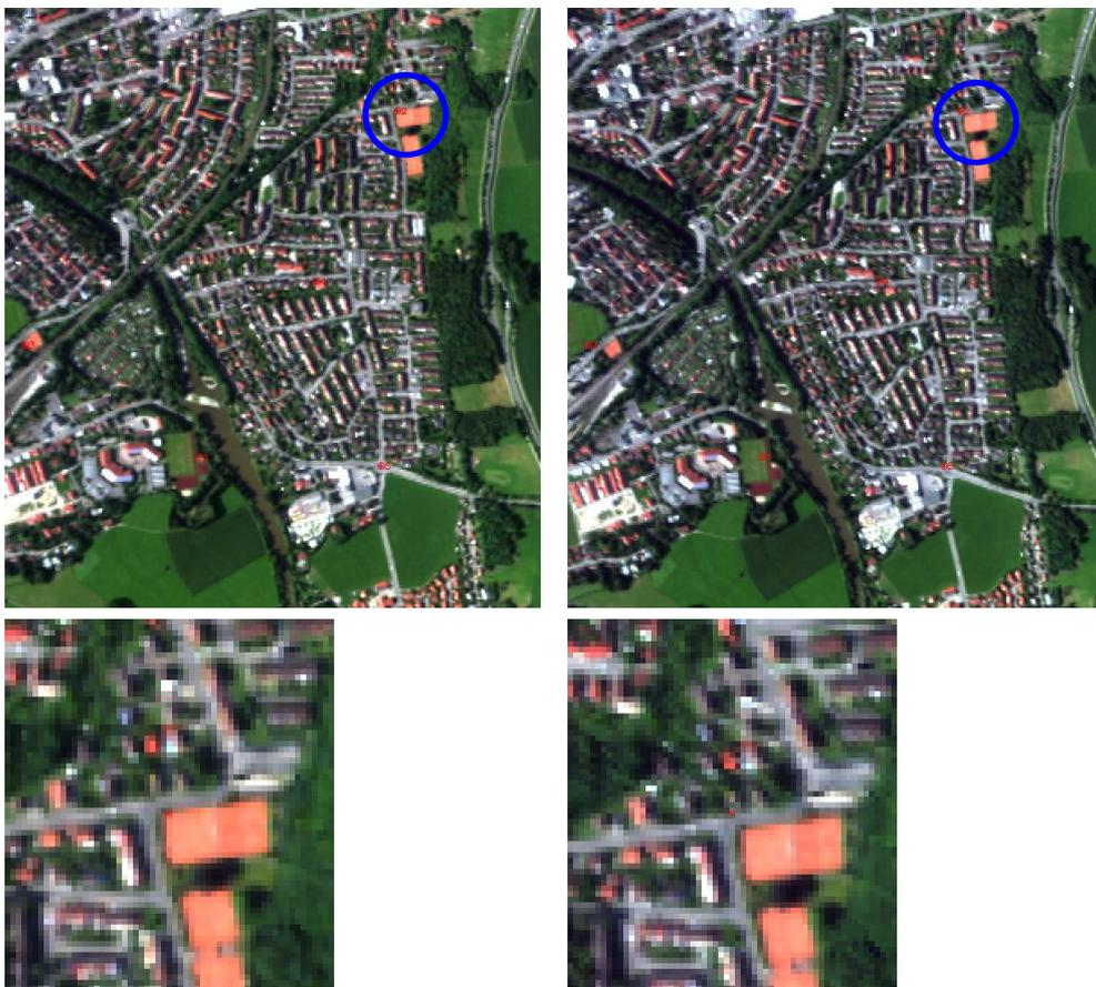
Figure 4: Results of geometrically corrected HyMap data (Kaufbeuren 2008) with PARGE (left) and ORTHO (right): Direct comparison.
