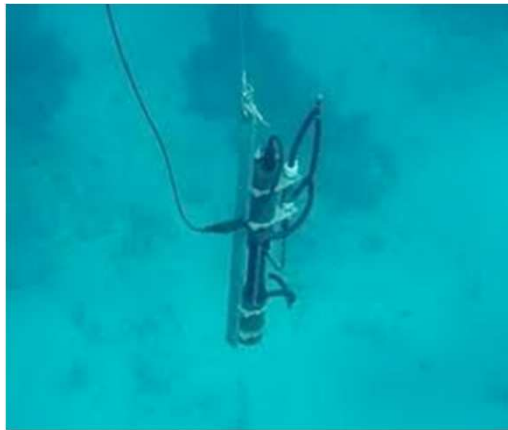
Wetlabs AC-S: hyperspectral absorption (a) and attenuation (c) [ b = c - a ]
